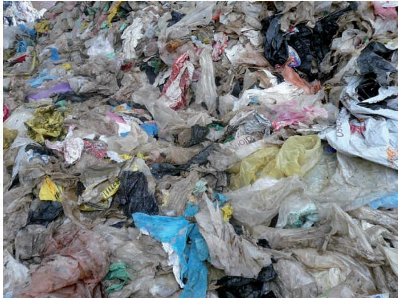
Fig. 2. Plástico film procedente de RCD/ Fig. 2. Plastic film produced from CDD.
