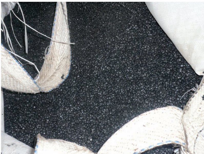
Fig. 1 Granza de polietileno obtenida a partir de residuos plásticos/ Fig. 1. Polyethylene chips produced from waste plastic.
