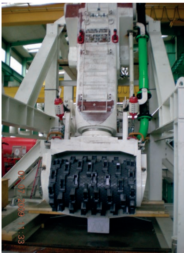
Fig.13. Cabezal convencional para suelos y rocas blandas/ Conventional head for soils and soft rocks.
